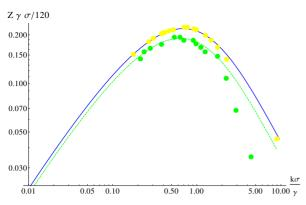
Figure 4: Space-charge impedance. ELEGANT-BH algorithm (green), analytical form Eq. 3 (blue), ELEGANT built-in LSCdrift element, very close to Eq. 3 (yellow).
