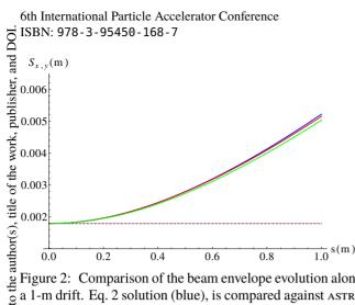
Figure 2: Comparison of the beam envelope evolution along a 1-m drift. Eq. 2 solution (blue), is compared against ASTRA (red), and ELEGANT-BH simulation (green). The dashed line attribution corresponds to no space-charge case.
