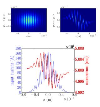
Figure 3: Modulated longitudinal phase space of a Gaussian beam before (top left) and after (top right) the application of one space-charge kick. Comparison of the induced energy modulation (bottom plot, red trace) computed from top-right image with the current distribution (bottom plot, blue trace).
