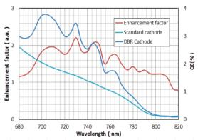
Figure 5: QE versus wavelength for photocathode samples with and without DBR. The QE enhancement factor is shown in red.
