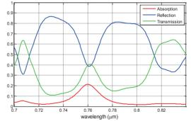
Figure 2: Calculation of absorption, reflectivity and transmission of a photocathode with DBR structure.
