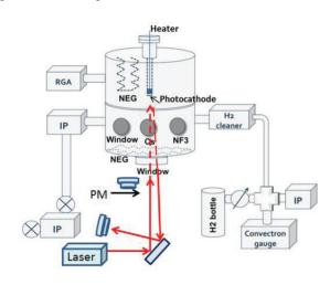
Figure 3: Schematic of the vacuum test chamber used to Theasure QE versus laser wavelength. IP: ion pump, measure QE versus laser wavelength. IP: 10n pump, NEG: non-evaoprable getter pump, PM: laser power meter. A schematic of the low voltage Mott polarimeter can be found in reference [5].
