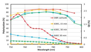
Figure 7: QE and polarization versus laser wavelength for DBR (in red) and standard strained-superlattice photocathodes studied in the micro-Mott apparatus (in, yellow, green and blue).
