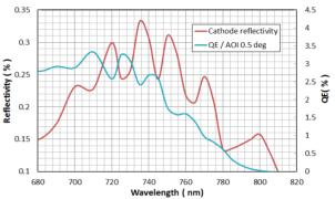
Figure 4: QE and photocathode reflectivity versus laser wavelength for a DBR photocathode sample. AOI: angle of incidence. Notice that QE peaks occur at reflectivity minima.
