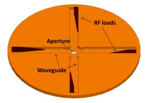
Figure 1: Geometry of single CLIC-G cell.
