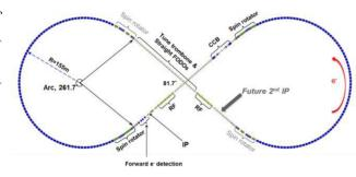
Figure 6: Geometric layout of the figure-8 shape electron collider ring with one IP and major machine sections.
