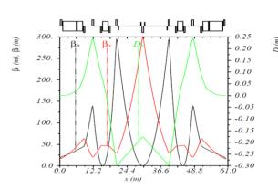
Figure 3: Optics of the Chromaticity Compensation Block (CCB) in the MEIC collider ring.
