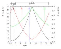
Figure 1: Optics of a normal arc FODO cell in the MEIC electron collider ring.
