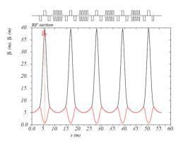
Figure 4: Optics of RF section in the MEIC electron collider ring.
