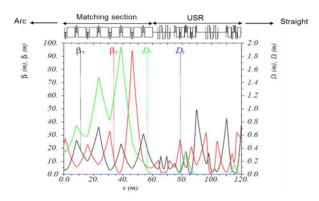
Figure 2: Optics of matching and USR sections in the MEIC electron collider ring.
