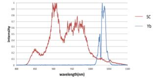
Figure 8: The spectrum of Yb fiber laser and SC light.
