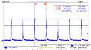
Figure 6: mode-locked pulses of Yb-doped fiber laser observed by using the oscilloscope.
