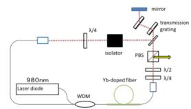
Figure 4: a mode-locked Yb-doped fiber laser setup.
