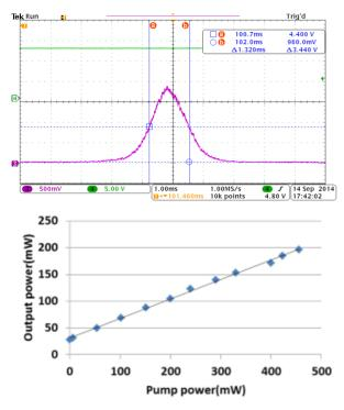
Figure 7: The stretched pulse observed by using the oscilloscope (top) and the relation of pump and output power (bottom).
