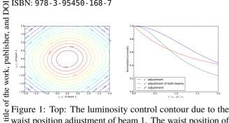
Figure 1: Top: The luminosity control contour due to the waist position adjustment of beam 1. The waist position of The other beam is intact. For the other beam is intact. For the other beam is intact. For the other beam and  $\beta^*$  tuning or both beams, the  $s_x^* = s_y^* = s^*$  and  $\Delta\beta^*$  is the beta function tuning in the both figures the luminosity is normalized by
