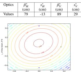
Figure 4: The luminosity reduction as function of the  $s_H^*$  and  $s_V^*$  of the blue beam. The requested  $s_V^*$  change is marked with blue dots; the requested  $s_H^*$  is marked with green dot and the origin  $s^*$  is marked yellow dot.
