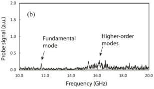
Figure 5: The rf spectrum of the signal picked up by a loop antenna at the periphery of the PBG structure: (a) the structure wrapped in foil; (b) the structure with 6 SiC absorbers.
