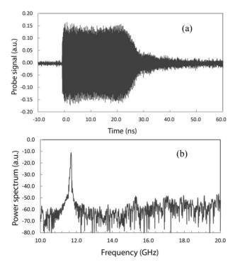
Figure 3: The rf signal in the downstream coupling waveguide of the PBG structure: (a) time-domain; (b) Fourier transform.
