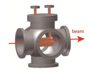
Figure 1: A 16-cell traveling-wave PBG accelerator structure with two waveguide couplers installed in a vacuum chamber for the wakefield tests.
