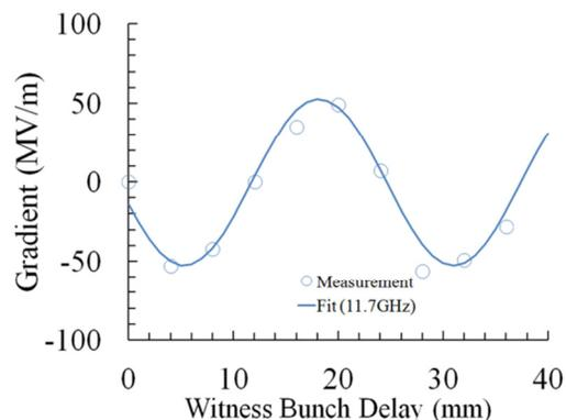
Figure 5: Accelerator gradient mapped out through the energy gain or loss of witness bunch at different delay positions in respect to the incident RF.
