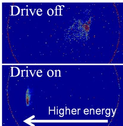
Figure 4: Acceleration of the witness bunch while the drive bunch train is on.
