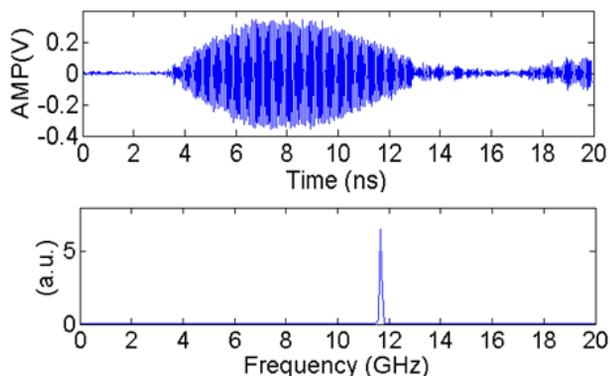
Figure 3: The measured rf pulse and its spectrum at output of the power extractor.
