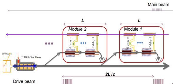
Figure 1: Two-beam acceleration staging using a fast kicker and high power RF delay lines.
