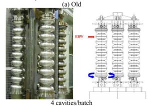
(b) New Figure 4: Welding of cavity.
