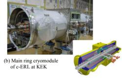
Figure 2: Cryomodules for c-ERL at KEK.
