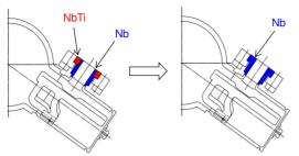
Figure 3: Nb Gr-2 flange of cavity.
