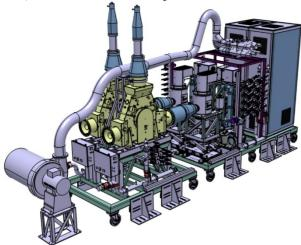
Figure 1: Tetrode based RF Module.
