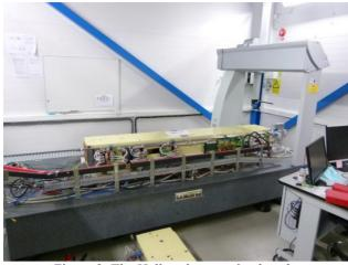
Figure 3: The Hall probe mapping bench.
