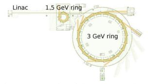
Figure 1: An overview of the MAX-IV accelerator complex. Courtesy of MAX IV Laboratory.
