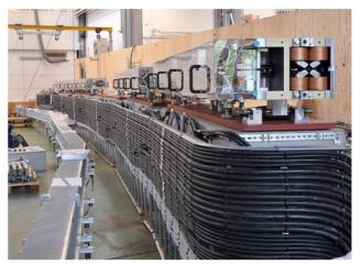
Figure 2: Image of one achromat (mock-up). Courtesy of MAX IV Laboratory.
