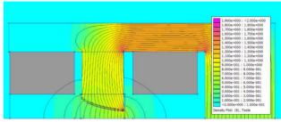
Figure 7: The cross section used for the FEMM calculations. The colour scale goes from 0 to 2 T.
