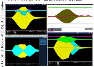
Figure 5: Scope signals during B=5 T run at ~11MV/m. <u>Top Left:</u> PU2, SPS upstream, SPS downstream, Light#3; <u>Top Right:</u> PU1, Faraday Cup, Light #1 and #2; <u>Bot. Left:</u> Forward and Reflected powers from Right and Left Coupler arms;
