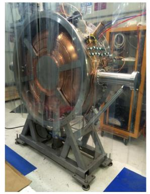
Figure 2: MICE Cavity in the MTA clean room, shortly after it was moved from Lab 6.
