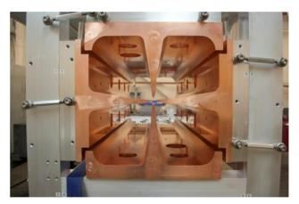
Figure 5: RFQ module in assembly fixture.
