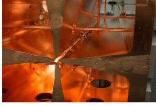
Figure 7: Brazed RFQ inner cavity
