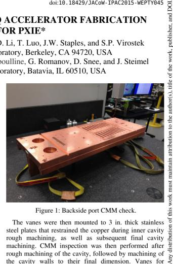
Figure 1: Backside port CMM check.
