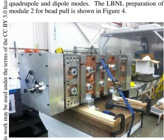
Figure 4: LBNL module 2 prep for bead pull.
