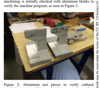
Figure 2: Aluminum test pieces to verify cutback machining program, if acceptable the program is saved on machine to be duplicated on the production part.
