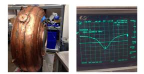
Figure 1: Cavity frequency measurement Left: Set up; Right: S11 measurement on Network Analyzer.
