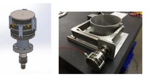
Figure 8: Left:the modified actuator design; right: the actu-ator functional test set up.
