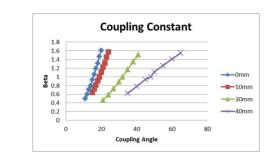
Figure 6: Omega3p simulation results: the coupling constant as a function of coupling angle with difference coupler loop positions.
