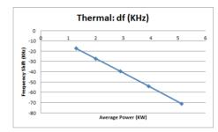
Figure 4: Frequency detuning due to thermal expansion.
