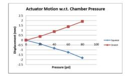
Figure 9: Functional test results of the modified actuator prototype.
