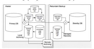
Figure 3: Database at sensor level (left) redundant DB at server level.
