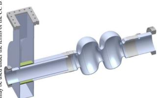
Figure 1: Cornell ERL injector cavity with symmetric coupler taken from [1]
