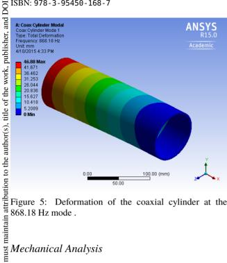
Figure 5: Deformation of the coaxial cylinder at the 868.18 Hz mode .
