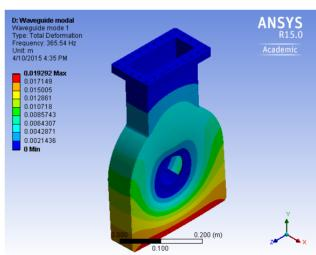
Figure 4: Deformation of the waveguide at the 365.54 Hz mode .
