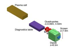
Figure 1: A 3D CAD image of the spectrometer system annotated with distances along the *z* direction from the exit of the plasma cell to the magnetic centres of magnets, and the centre of the scintillator screen.
