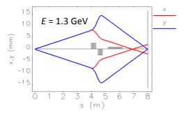
Figure 4: ELEGANT [11] simulation results showing the trajectories of electrons with angles at the plasma cell of  $\pm 2$  mrad. The first quadrupole has  $K_1 = +4.07$  m<sup>-2</sup> and the second quadrupole has  $K_1 = -4.07$  m<sup>-2</sup>.
