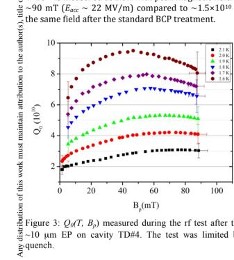
Figure 3:  $Q_0(T, B_p)$  measured during the rf test after the ~10 µm EP on cavity TD#4. The test was limited by
