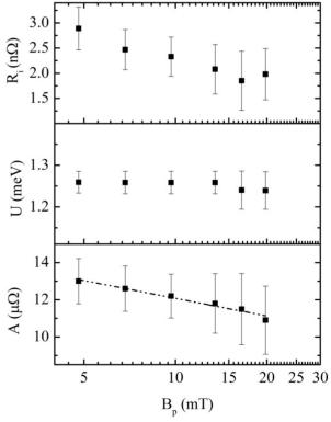
Figure 2: Dependencies of  $R_i$ , U and A on  $B_p$  from the fitting of Eq. (1) with the method described in Ref. [9] on the amplitude of the peak magnetic field for cavity TD#4 after 10 µm EP. The dashed line in the plot is a linear fit of  $A[\ln(B_n)]$ .
