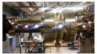
Figure 5: Pill box cavity with plasma.
