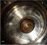
Figure 4: Niobium samples and electrode in the pill box
