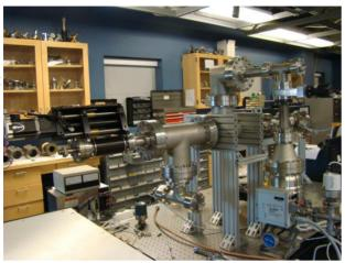
Figure 1: Cylindrical cavity with moving inner electrode for processing experiments.
