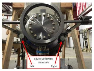
Figure 4: Dial indicators for deflection measurements.
