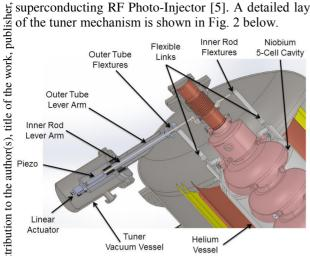
Figure 2: Detail design of mechanical tuning system.
