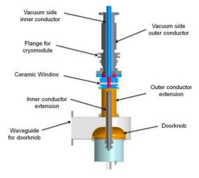
Figure 1: Fundamental power coupler design layout.
