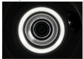
Figure 6: 5-cell cavity RF surface after BCP.
