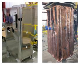
Figure 8: Magnetic and heat shields. 7: Accelerator Technology **T07 - Superconducting RF**
