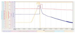
Figure 3: Pressure spike during cavity quench is clipped by automatically opening the warm GHe return valve.
