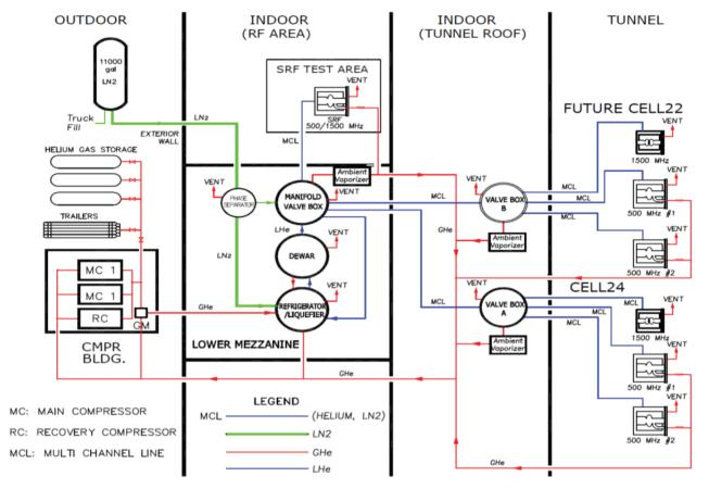
Figure 1: RF cryogenic plant diagram.
