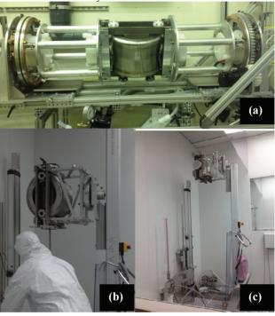
Figure 3: (a) DQWCC on the BCP equipment at ANL; (b) Setup the HPR at ANL; (c) DQWCC after HPR.
