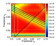
Figure 12: Tune scan of luminosity for LER with crab waist. The black lines indicate various resonances.
