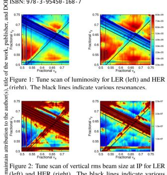
Figure 1: Tune scan of luminosity for LER (left) and HER (right). The black lines indicate various resonances.
