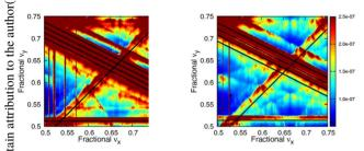
Figure 2: Tune scan of vertical rms beam size at IP for LER (left) and HER (right). The black lines indicate various must resonances.
