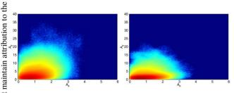
must Figure 8: Beam tail simulated by SAD for a baseline lattice of LER without (left) and with (right) ideal crab waist.
