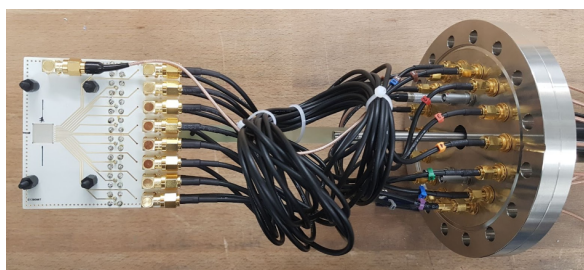
Figure 5: Prototype T0 detector build for the mCBM experiment. The diamond sensor is bonded on a PCB which is pneumatically driven into the beam-line in front of the target.
