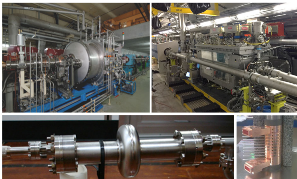
Figure 1: Difference crab cavities fabricated and operated. Top left: Squashed crab cavity at 509 MHz operated in the HER ring @ KEK. Top right: Double Quarter Wave crab cavity at 400 MHz operated in the SPS ring @ CERN. Bottom left: Single-cell prototype of the 3.9 GHz 9-cell crab cavity for ILC. Bottom right: 12-cell copper travelling-wave structure for crabbing in CLIC.
