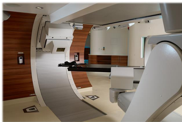
Figure 7: Gantry room: automatic patient positioning system and rolling floor. Gantry at 60°, beam entry from left.
