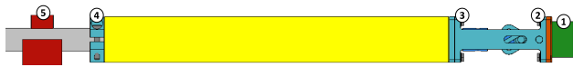
Figure 6: Detail of the CAD model of the heating setup. The numbers 1 – 4 indicate the position of the temperature sensors. Position 5 shows a part of the manipulator axis (gray) and optional passive cooling clamps (red).
