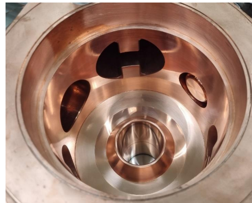
Figure 2: Inner view of the cavity body. Courtesy of VITZRO TECH.
