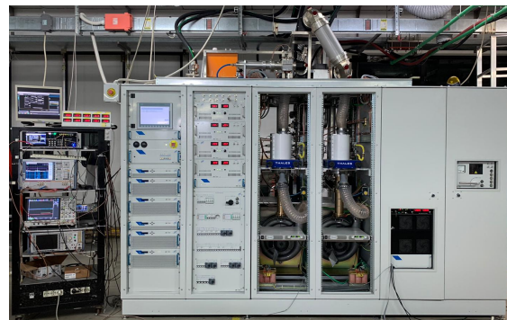
Figure 1: FAT setup. The six-racks RFPS is shown with the middle covers removed, revealing the twin cavities configuration. On the far left, the rack of the required instruments.
