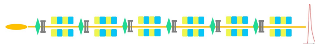
Figure 2: Layout of the undulator system. Six undulator segments are used for SASE amplification to saturate at the typical wavelength.
