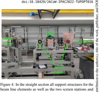
Figure 4: In the straight section all support structures for the beam line elements as well as the two screen stations and the dipole to separate electron and THz beam are installed and aligned. The bellows and beam pipes connecting the undulator and the beam dump are ready for installation. The dispersive section with the high power beam dump is currently in production.
