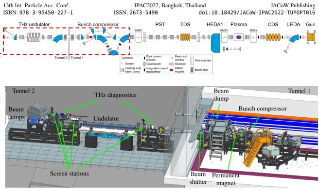
Figure 1: Schematic overview of the complete PITZ beam line (top). The beam line extension for the THz@PITZ project is surrounded by the red dashed box, while the CAD model of the beam line extension is shown in more detail in bottom of the figure.
