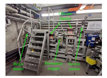
Figure 2: Picture of the finished beam line installations in tunnel 1. The last two dipoles of the bunch compressor chicane, the chicane screen station, the permanent magnet and the beam shutter are highlighted. The other elements, e.g. the collimator and another screen station are covered by the ladder system, which is on top of the new beam dump.
