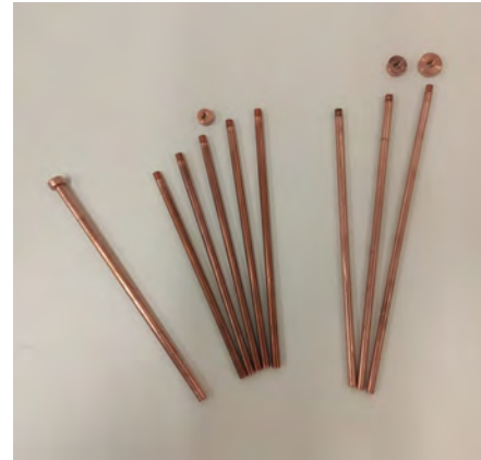
Figure 1: Dummy parts on the right were tested to achieve critical coupling strength at room temperature. Center dummy components are of similar dimensions to the previously installed coupler on the left and were used to determine the required length adjustment.
