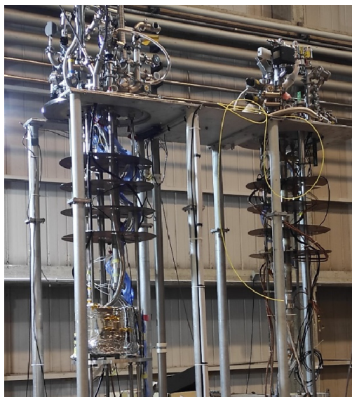
Figure 4: LASA VT inserts. On the left the one in use for PIP-II cavities equipped with tube-in-tube heat-exchanger (wrapped in MLI) and Joule-Thomson refilling system.
