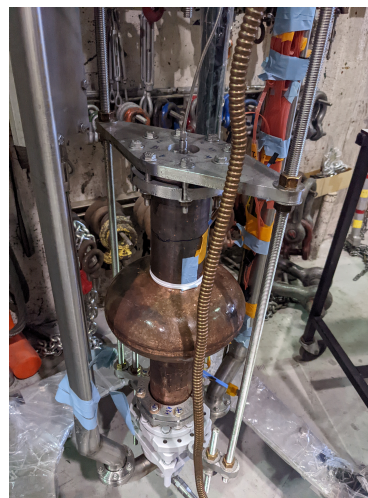
Figure 1: SN 38-39 cavity on the RF testing insert under vacuum.
