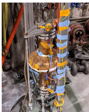
Figure 6: SN 4 cavity on the testing insert under vacuum.
