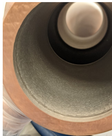
Figure 9: Image of the Nb 3 Sn coating at the inner surface of RF test cavity SN 4 and location where dust residue was noticed upon removal of the RF test insert.
