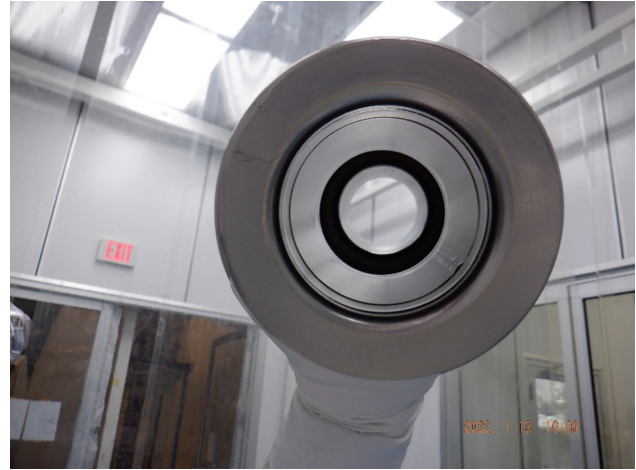
Figure 8: Nb_3Sn coating on the LR1-3 reentrant cavity.
