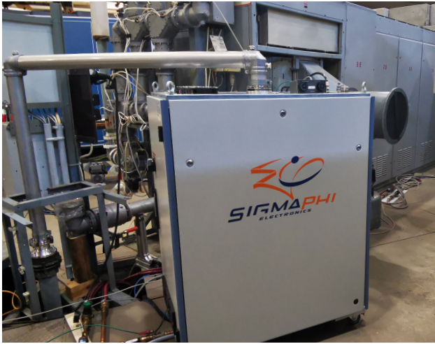
Figure 2: Image of the solid state RF amplifier with connected coaxial line in front of the former klystron rack gallery.
