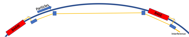
Figure 1: A conceptual overview of the experiment shown along the northern arc of the CESR ring. In the diagram, positrons circulate the ring clockwise, west to east. The light (yellow) from dipole B44W is propagated to the east where it is interfered with light from B46E. The diagram is not to scale.
