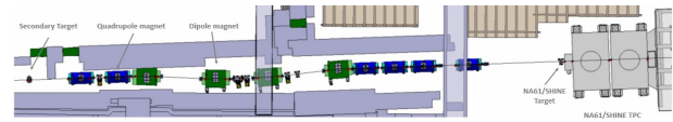
Figure 7: A CAD drawing of the low-energy branch of the H2 line, starting at the secondary target and ending at the NA61/SHINE TPC.
