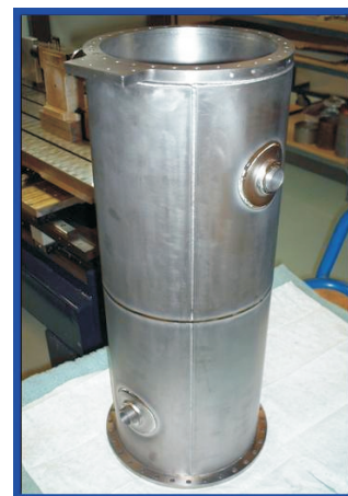
Figure 5: The first superconducting cavity produced by PAVAC Industries: the 141MHz quarter wave bulk niobium resonator for the ISAC-II linac upgrade.
