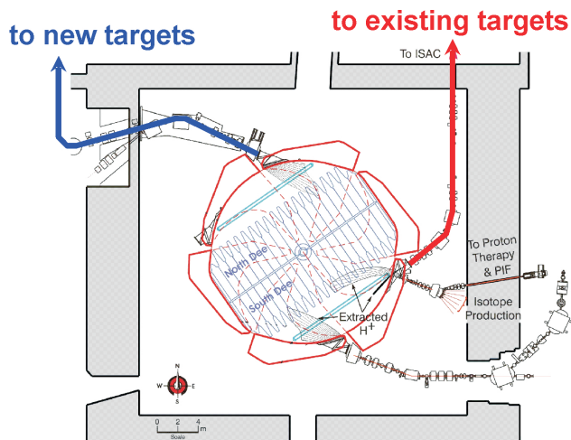
Figure 2: Schematic of the TRIUMF cyclotron. Three operating extraction beam lines in the SE side. One existing extraction beam line in the NW side.
