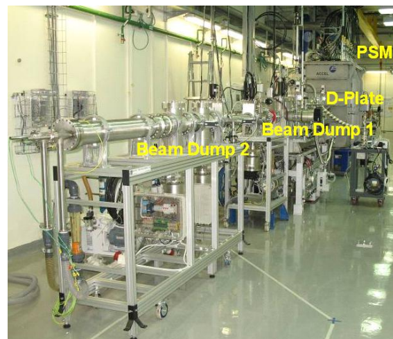
Figure 2: Downstream view of Phase I of SARAF. From right to left: PSM, Diagnostic plate (D-Plate), low power (Beam dump 1, copper, 6 kW) and high power (Beam dump 2, tungsten, 20 kW) beam dumps.
