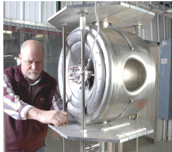
Figure 5. First SC Spoke Cavity prepared for vertical test.
