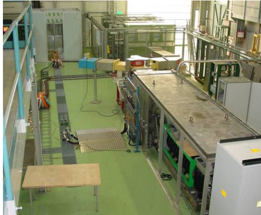
Figure 6: The Test Stand with klystron and modulator (right), ion source cage (top).
