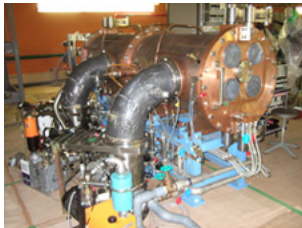
Figure 5: Photograph of the four-rod RFQ settled in the RIBF building for high power tests.
