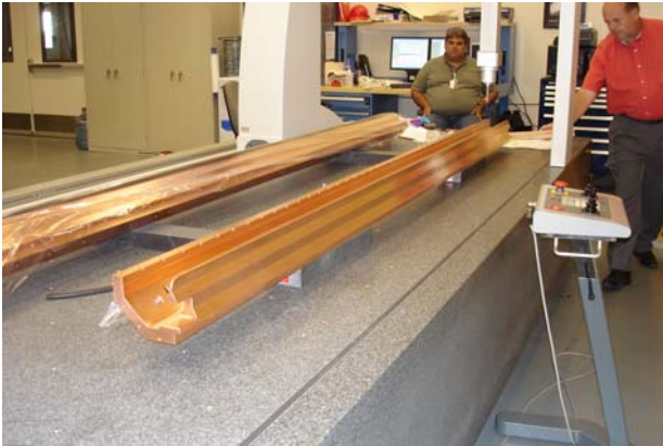
Figure 2: CMM measurements of the univane at SLAC.
