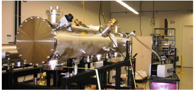
Figure 4: RFQ in the vacuum chamber.
