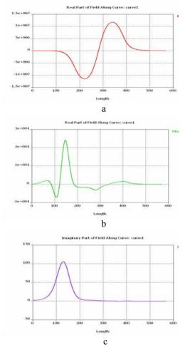
Figure 2: Longitudinal (a), transverse (b) components of electric field and transverse component of marmagnetic field (c) on structure axis for electric wall boundary condition.
