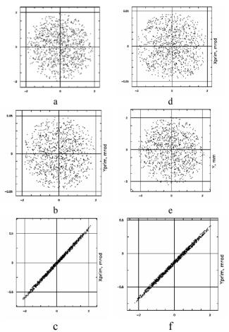
Figure 3: Beam parameters before (a - cross-section, b - phase plane x-xp, c- phase plane y-yp) and after passing the accelerator (d- cross-section, e - phase plane x-xp, f - phase plane y-yp).
