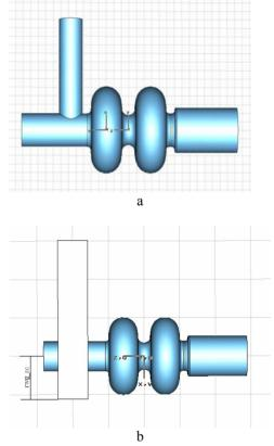
Figure 1: Coaxial and waveguide input couplers.
