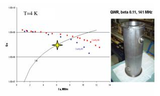
Figure 1: Vertical cold test results of the two first QWR prototypes. Yellow star: ISAC-II, phase 2 specifications.
