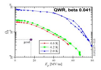
Figure 5: Vertical cold test results of the beta 0.041 QWR for the Re-Accelerator.
