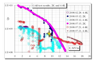
Figure 9: Vertical cold test results of the beta 0.22 Single-Spoke prototype.
