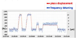
Figure 11: Frequency variation (blue dots) while moving the piezo-tuner (red dots).
