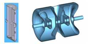
Figure 10: 176 MHz, beta 0.15, HWR (left) and 352 MHz, beta 0.30, Triple-Spoke cavity (right) for the EURISOL driver.
