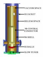
Figure 4: Stainless Steel balls (in red) inserted inside the inner conductor to damp mechanical vibrations.
