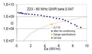
Figure 3: Vertical cold test results (T=4K) of the first QWR for the PIAVE-ALPI upgrade.
