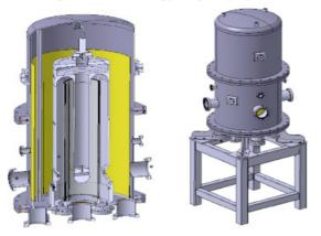
Figure 6: Sputtering chamber.
