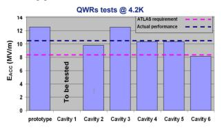
Figure 2: Vertical cold test results of the QWRs composing the new cryomodule for the ATLAS upgrade.
