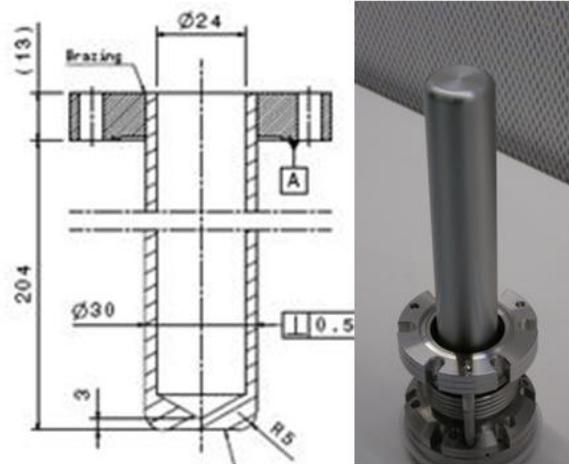
Figure 1: Picture and sketch of the plunger.
