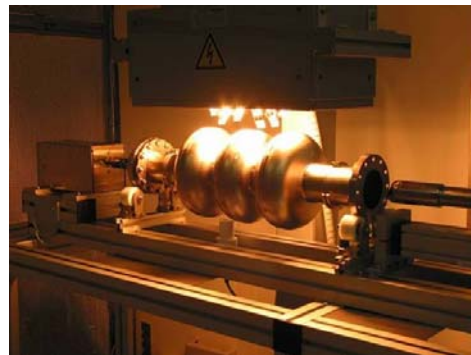
Figure. 2: 3-cell cavity assembled to the horizontal cleaning setup with IR-heater above the cavity
