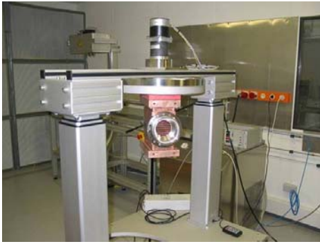
Figure 8: Waveguide assembled to the vertical cleaning setup.
