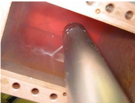
Figure 9: Nozzle and CO 2 - jet inside waveguide.
