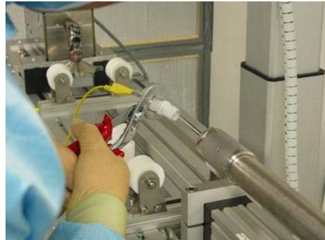
Figure 6: CO 2 cathode cleaning by hand.
