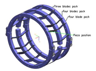
Figure 3: Improved blade tuner design with the upgraded blade positions and distribution.
