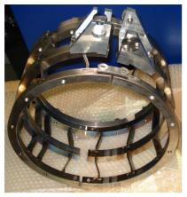
Figure 4: One of the Blade Tuner manufactured for ILCTA NML facility at Fermilab.
