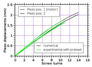
Figure 5: Tuning range results for ILCTA tuner, experimental vs. simulation at room temperature.
