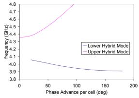
Figure 1: The modal distribution of the first two dipole passbands in the ILC Crab cavity.
