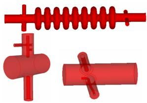
Figure 2: Model of the ILC deflecting mode cavity.
